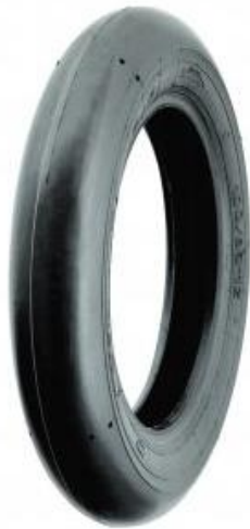
A race tyre for Vespas: Heidenau Slick 3.50-10 TL NHS
